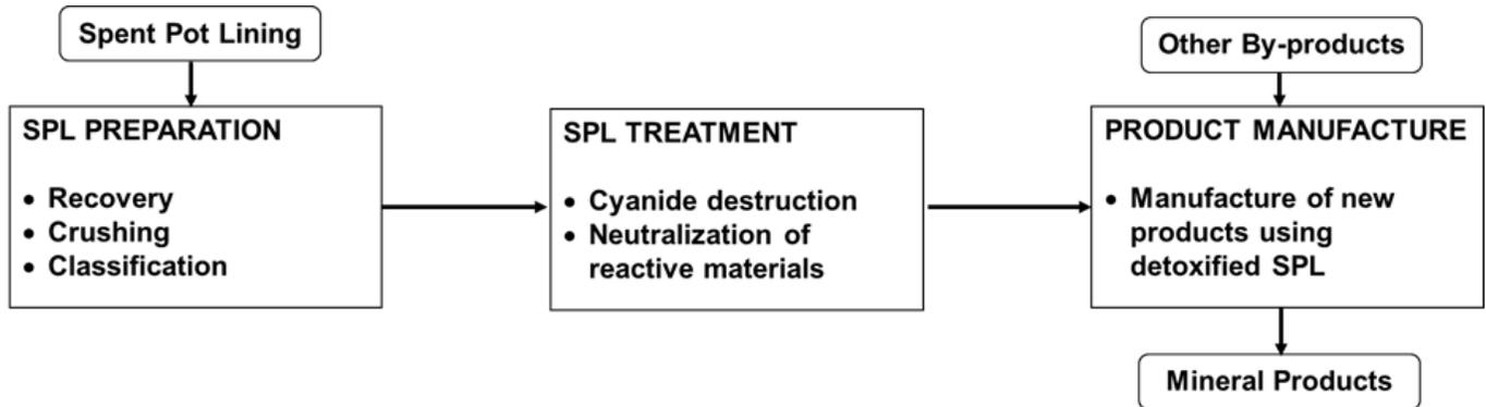
Figure 2 SPL Processing Flow Diagram
